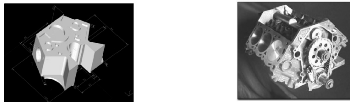
Figure 4 - Cylinder block used in reconfiguring process plans and a geometric model of one of its family members (2 cylinders engine block) (Azab et al., 2006).
